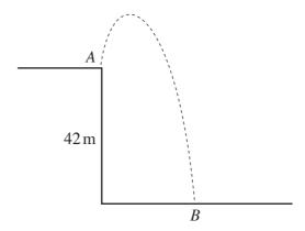
The horizontal and vertical components of the stone's initial velocity are  $4.5\,\mathrm{ms}^{-1}$  and  $22.4\,\mathrm{ms}^{-1}$  respectively.
