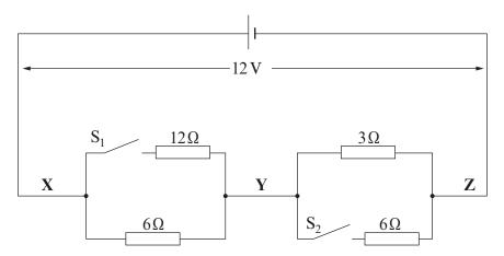
(i) Calculate the resistance of the circuit when both  $S_1$  and  $S_2$  are closed. [3]
