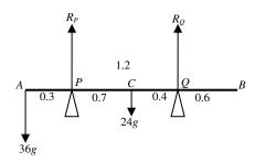
Moments about P M1dim correct equation All forces, no extra  $36g \times 0.3 + R_O \times 1.1 = 24g \times 0.7$ **B**1 any correct moment **A**1 correct equation  $R_Q = 53.45 \text{ (N)}$ **A**1 cao Resolve vertically dim correct equation M1All forces, no extra **A**1
