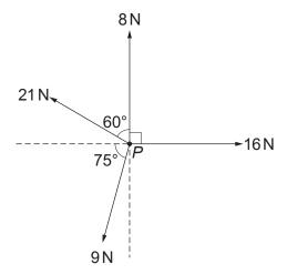
Calculate the magnitude of the resultant of the forces acting at *P*. Determine the angle the resultant makes with the 8 N force. Give your answers correct to one decimal place. [8]
